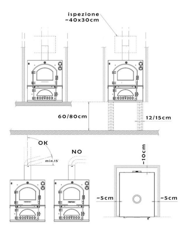
**OBSERVATION:** To facilitate the flue draft, it is a good idea to connect a flue with an inclination of at least 15°. As can be seen in the drawing, it is advisable to avoid connections with a 90° connecting curve.
